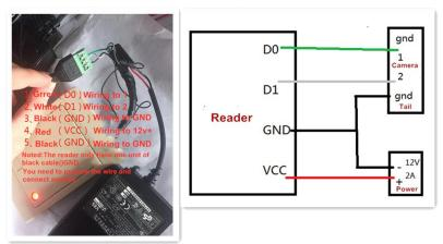
2. Face recognition machine wiring for face access by access controller solution
