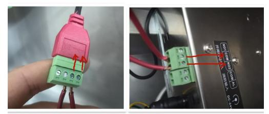
1.Connect the switch symbol from the red 4 pin cable to the turnstile gate main board no2 and com(Right Open)
