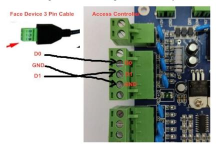
3.. Face recognition machine wiring for face directly open the turnstile or electric lock
